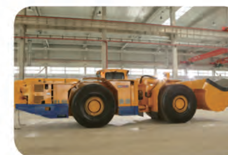
混合动力铲运机 Hybrid LHD of model AHCY514, a innovative product of biggest LHD weigh with 14 tons load
