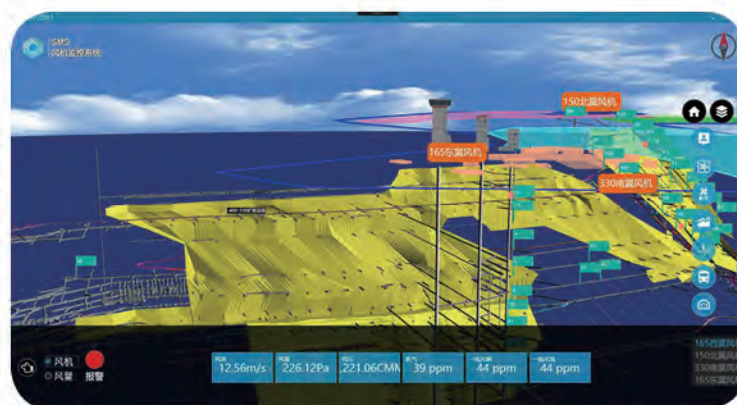
三维管控平台 Three-dimensional control platform
